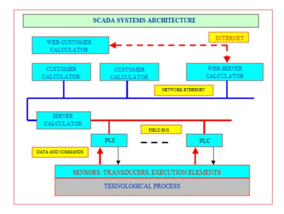
Fig.2. SCADA systems architecture
