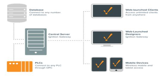
Fig. 3. Ignition SCADA Architecture
